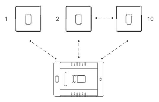
Max. 10 Kinetic Switches to pair ONE Dimmer Receiver.
