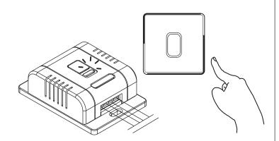
While the indicator on receiver flashes, press the Kinetic switch ONCE to complete the pairing.
