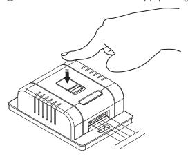
Press the Pairing Key for 10-12s, untill the Red indicator changes into Blue light.
