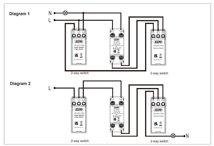
This intermediate ON/OFF switch is suitable for 3-way lighting circuits. There are four terminals, L1 load 1, L2 load 2. Please follow the wiring instructions.
