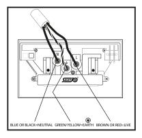
**5.** If you are fitting your converter switched socket outlet into a metal wall box, then you MUST make an earth connection between the converter switched socket outlet and the metal wall box. Use Green / Yellow sleeved earthing cable.
