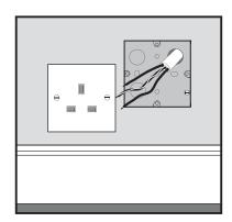
**3.** Ensure that there is sufficient length of cable tail to enable easy wiring and not too much to make losing the excess length in the back of the socket too difficult. Tighten the screw terminals onto the exposed wires maintaining correct polarity using the easy to follow wiring diagram.
