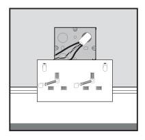
**4.** Remove fixing screws and cover caps that are housed inside the back of your converter socket. Screw the 2 screws through the holes located in the front of your converter socket and into the threaded holes provided in the wall box and tighten sufficiently to hold the converter socket in place. Do not overtighten.
